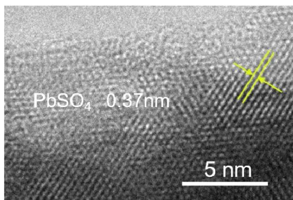
**Fig. S4** TEM image of the perovskite precursor solution with  $\text{Rb}_2\text{SO}_4$  additive.
