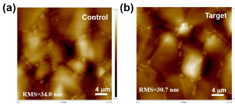
**Fig. S6** AFM images of perovskite films (a) without and (b) with  $\text{Rb}_2\text{SO}_4$  additive.
