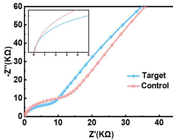
Fig. S15 Nyquist plots for the control and target devices.
