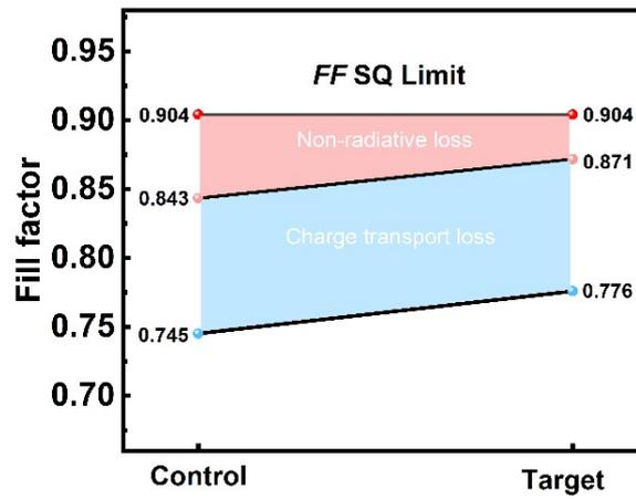
**Fig. S19** The  $FF$  loss of devices, where blue, pink, red balls correspondingly represent the measured  $FF$ ,  $FF_0$  (without charge transport loss) and  $FF_{S-Q}$ .
