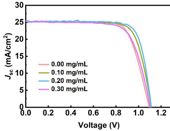
**Fig. S18** The  $J$ - $V$  curves of PSCs with different concentrations of  $\text{Rb}_2\text{SO}_4$  additive.
