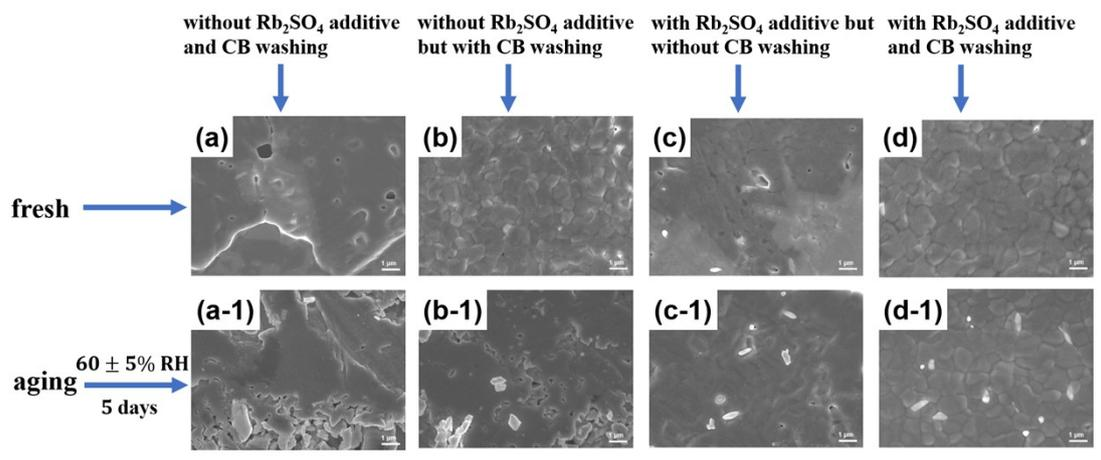
**Fig. S25** Top-view SEM images of the perovskite films before and after aging.
