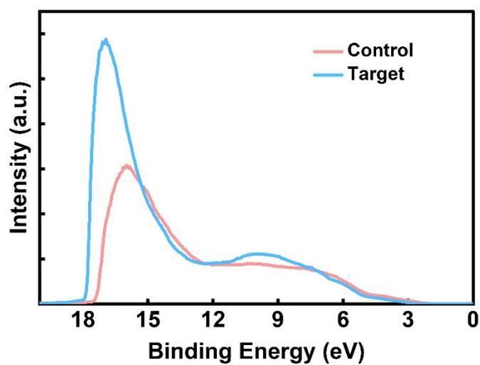
**Fig. S13** Ultraviolet Photoelectron Spectroscopy of the perovskite films.
