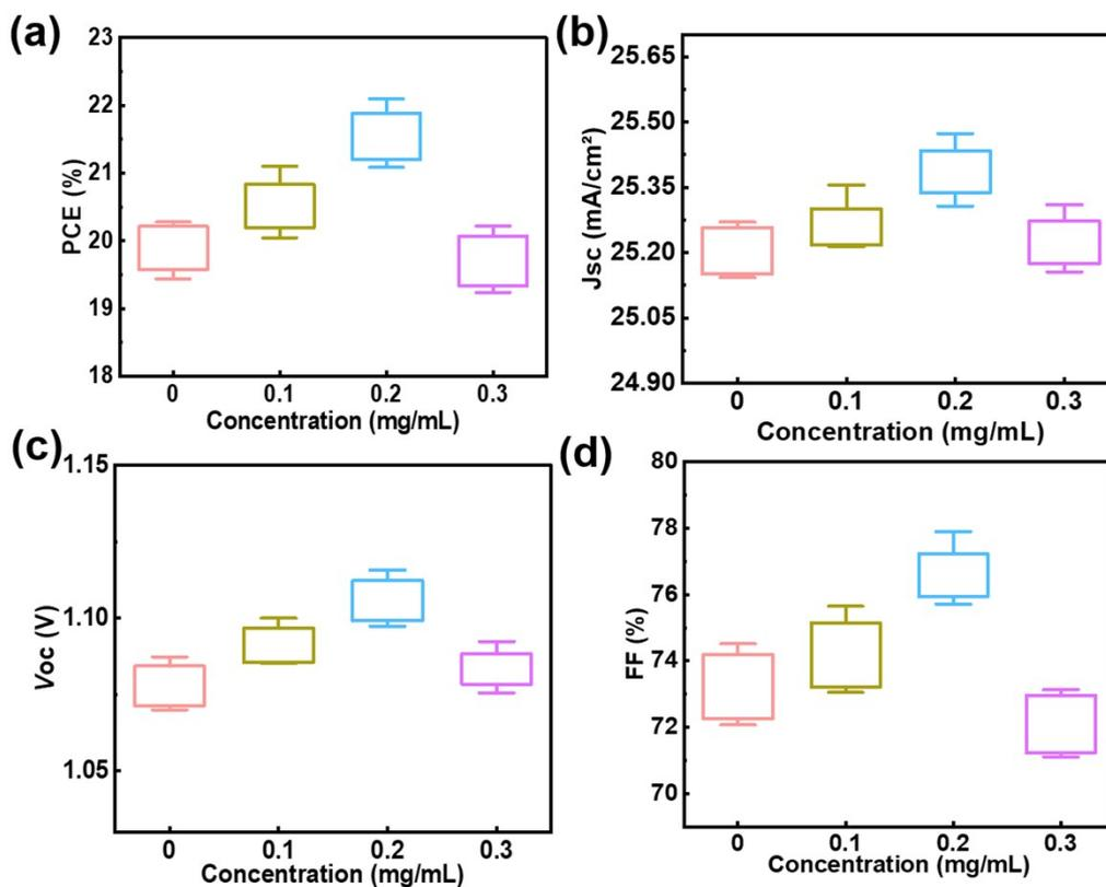
Fig. S17 Box charts of a) PCE, b)  $J_{sc}$ , c)  $V_{oc}$  and d) FF of the PSCs with different concentrations of  $Rb_2SO_4$  additive.
