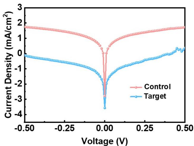
Fig. S16  $J - V$  curves for the control and target devices in the dark condition.
