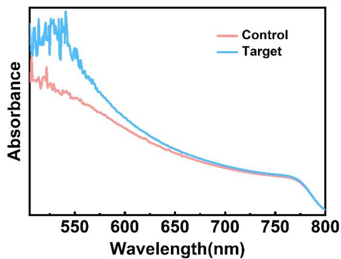
**Fig. S7** UV-visible absorption spectra of perovskite films without and with  $\text{Rb}_2\text{SO}_4$  additive.
