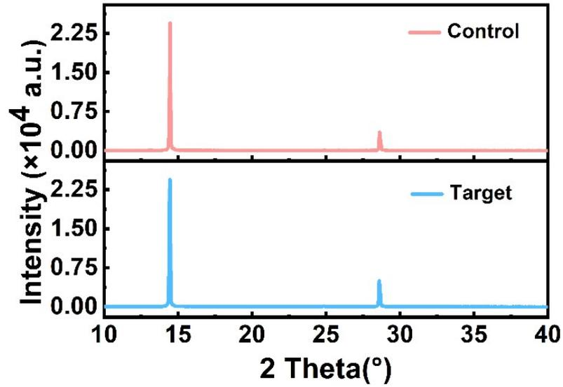
Fig. S8 XRD patterns of perovskite films without and with  $\text{Rb}_2\text{SO}_4$  additive.
