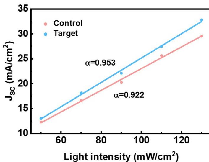
**Fig. S11**  $J_{\text{SC}}$  dependence on light intensity for the control and target devices.
