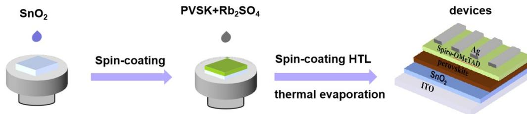
**Fig. S1** The preparation process of perovskite solar cells.
