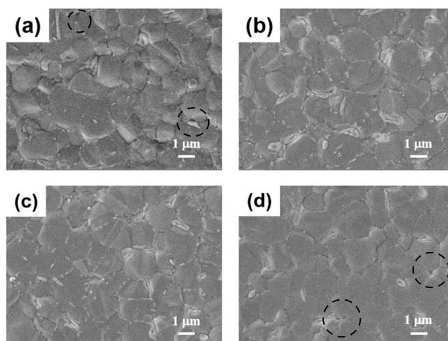
**Fig. S5** Top-view SEM images of the perovskite films with different concentration of  $\text{Rb}_2\text{SO}_4$  additive: (a) 0.00 mg/mL, (b) 0.10 mg/mL, (c) 0.20 mg/mL, and (d) 0.30 mg/mL, respectively.
