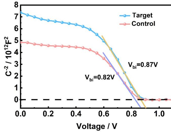
Fig. S14 Mott-Schottky curves of the control and target devices.
