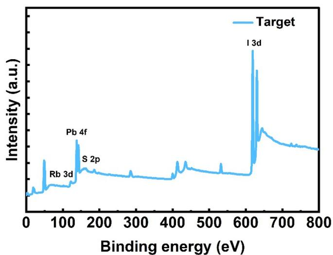
**Fig. S2** The full XPS spectra of the perovskite film with  $\text{Rb}_2\text{SO}_4$  additive.
