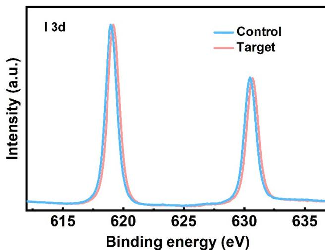
**Fig. S3** I 3d for control and target perovskite films.
