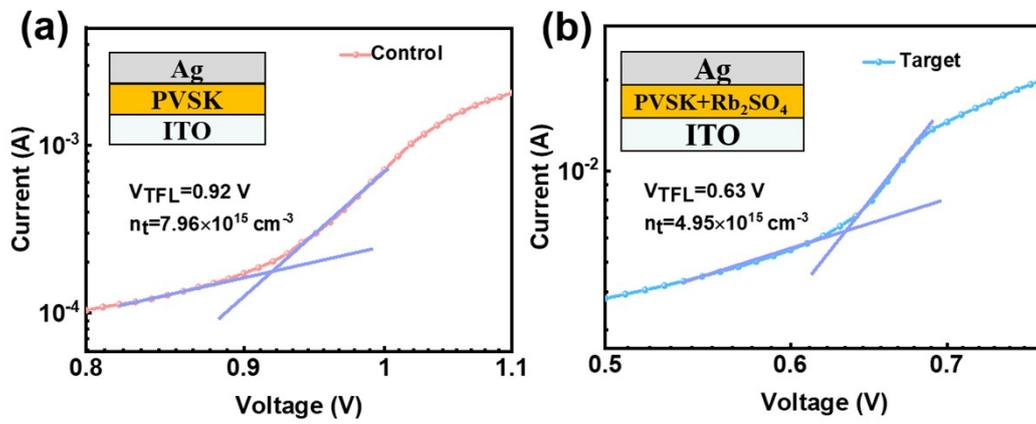
Fig. S9 The space charge limited current curves of the control and target devices.
