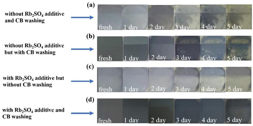
**Fig. S24** Moisture stability of the perovskite films with different preparation condition exposed to a relative humidity of  $60 \pm 5\%$  RH at the room temperature.
