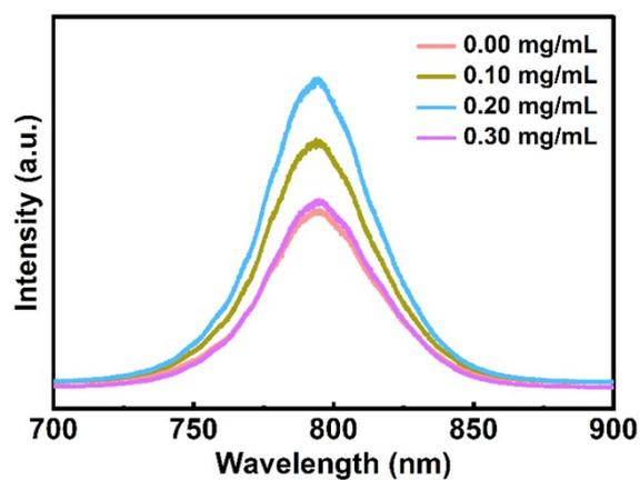
**Fig. S10** Steady-state PL spectra of the perovskite films with different concentration of  $\text{Rb}_2\text{SO}_4$  additive: 0.00 mg/mL, 0.10 mg/mL, 0.20 mg/mL, and 0.30 mg/mL, respectively.
