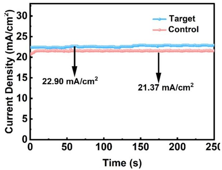
**Fig. S21** The steady-state current density at the maximum power point for the control and target devices.
