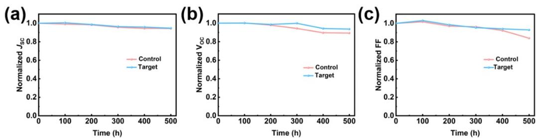
**Fig. S22** a)  $J_{sc}$ , b)  $V_{oc}$ , and c) FF versus time for the unencapsulated control and target devices aged in the air with relative humidity of 15 %-20 % RH in the dark at the room temperature.
