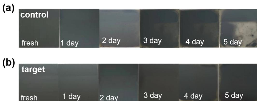
**Fig. S23** Moisture stability of the perovskite films a) without and b) with  $Rb_2SO_4$  exposed to a relative humidity of 50 %-60 % RH at the room temperature.
